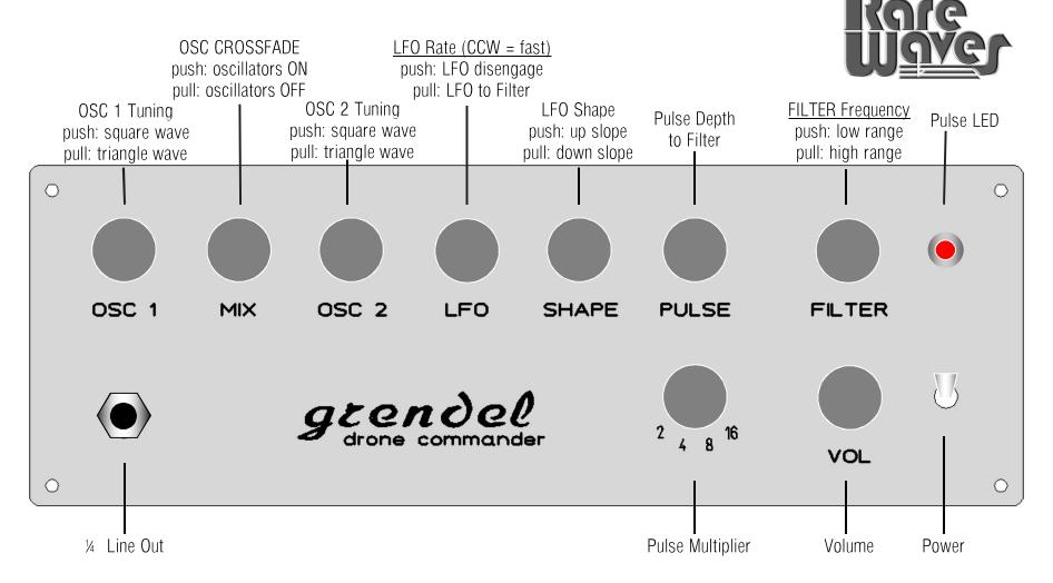
Two manually-tuned triangle/square wave oscillators with crossfade mixer Variable shape LFO (sawtooth pulse) with up/down slope control Pulse modulation, auto-synchronized to LFO at 2x, 4x, 8x, or 16x *via* phase-lock loop (PLL) A super-crusty voltage-controlled filter, modulated by LFO and Pulse; self-oscillates in low range Powered by 9V battery or included 9VDC adapter (2.1mm center pin positive)
