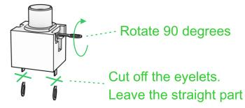
Place the jacks on the PCB with the side lead facing toward the TN mark printed on the PCB.
